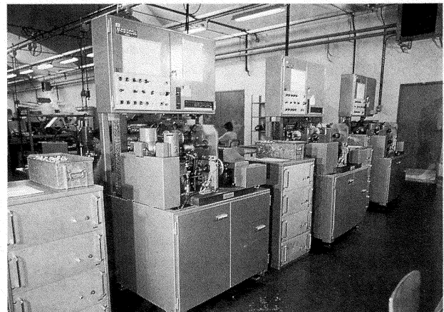
Partial view of the winding department for the production of film capacitors
