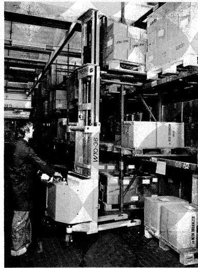
Fork lift truck 'ORMIC 10' Mod. W 10-36 P-Triplex
